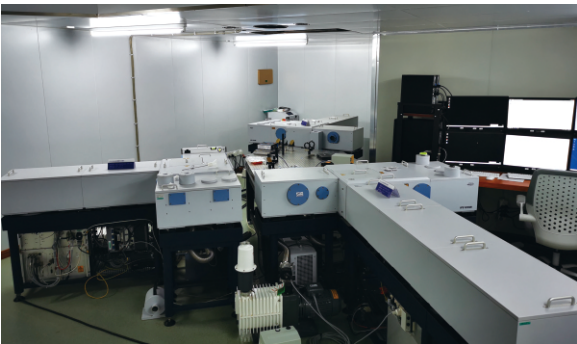
傅里叶变换红外光谱仪 (Bruker IFS 125HR)
